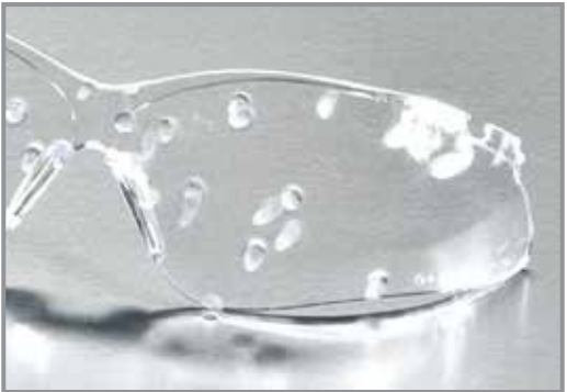
Ballistic Shooting Glasses withstand hits from 12-gauge, #4 steel shot at 20 yards.
