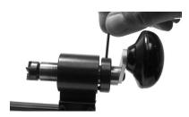
4. Loosen the two 6/32" SHCS with a 7/64" hex wrench that secure the Case Holding Collet assembly to the Base. This allows the Collet Assy to be moved to the right.
