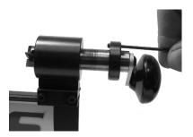
3. Slide the Adjustment Bushing towards the Cutter roughly ½" and temporarily lock it in place with the 8-32 SHSS.
