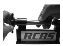
2. Adjust the 8-32 SHSS Adjustment Bushing Stop so that approximately 1/8" is exposed to the left of the Adjustment Bushing.
