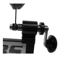
4. There are two case holding diameters machined into the case holder Collet. The smaller diameter is for the .408 CheyTac® and the larger diameter will accommodate the .416 Barrett® and .50 BMG.
