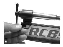
5. Slide the Cutter Assy to the LEFT until the Adjustment Bushing Stop is up against the Cutter Sleeve. Holding the Stop in position, slide the Case Holder assembly to the RIGHT, until the case mouth contacts the Cutter. Secure the two 6/32" SHCS to lock the Case Holder Assembly into place.
