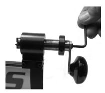
3. Select one of the three included Pilots for the cases you are about to trim. Install the desired Pilot into the Cutter Head and secure the 8-32 Socket Head Set Screw with a 5/64" hex wrench (not included).
