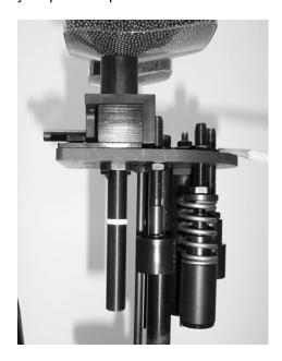
Hole in the middle of the crimp – not enough crimp start. Adjust Crimp Start die down in ¼ turn increments until desired crimp is achieved.
