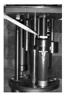
**Crimp Start adjustment:** This is an up or down adjustment. Adjusting the amount of crimp start will control the "hole" in the center of the loaded round. Too little crimp start will leave a hole that shot may spill out of. Too much crimp start can cause a "swirl" in the center of the crimp or cause a "buckle" near the top of the loaded round.
