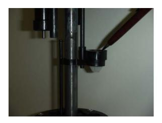
• Install Wad Holder Cap. Place cap on the Wad Holder and turn counter clockwise to lock in place.
