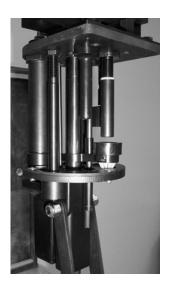
**Station 2**Priming: Primers are inserted manually, the hull is placed in the station and primers are seated by "feel". Full cycling of the handle is not achieved at this station.
