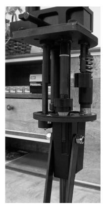
**Station 7** Empty, allows for the installation of an optional Taper Crimp die assembly.
