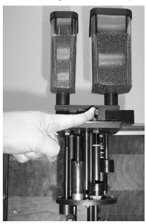
**Station 4**Wad Seating and Shot Charge: Insert wad into Wad Guide and cycle handle to the down position. The wad is seated into the hull. Slide the Charge Bar Handle to the left to dispense the shot charge.
