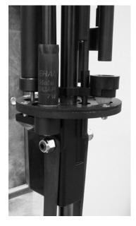
**Station 3** Powder Charge: Powder is dispensed into the hull by sliding the Charge Bar Handle to the right.
