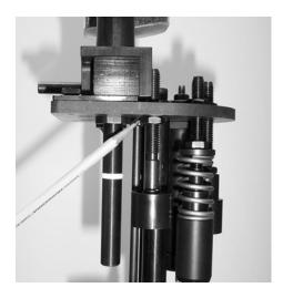
Concave crimp – not enough spring pressure. Adjust nut above the spring to increase spring pressure at station 6. Peaked crimp – wad not seated deeply enough or too much spring pressure at station 6.
