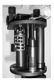
Inconsistent shot charges or shot dispenses when the Charge Bar Handle is cycled to the left. This is a bridging issue. Typically too large a size shot is being used. Shot larger than #5 requires the Steel Shot Conversion.
