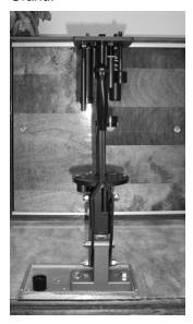
**Step 2** Install Hopper/Charge Bar assembly onto press frame. Place assembly onto top of press frame and attached with Thumbscrews provided.
